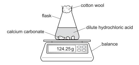
The mass of the flask and contents was recorded every 30 seconds. When the reaction stopped there were still small pieces of calcium carbonate in the flask.
