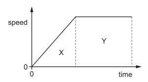
Which area represents the distance travelled while the car is accelerating?
