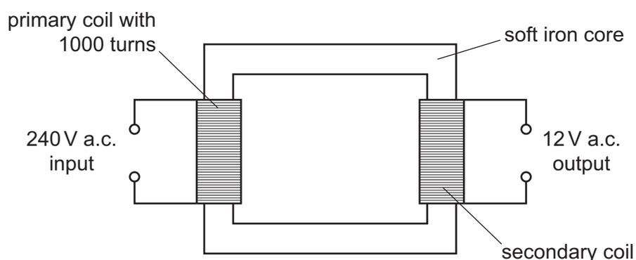
How many turns of wire are in the secondary coil?
