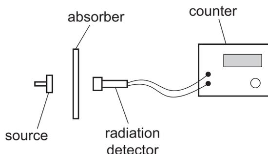
When a piece of paper is used as the absorber, the count rate drops to the background count rate.
