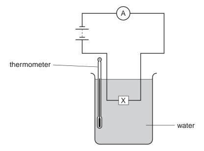
When the temperature of the water is increased, the reading on the ammeter increases.
