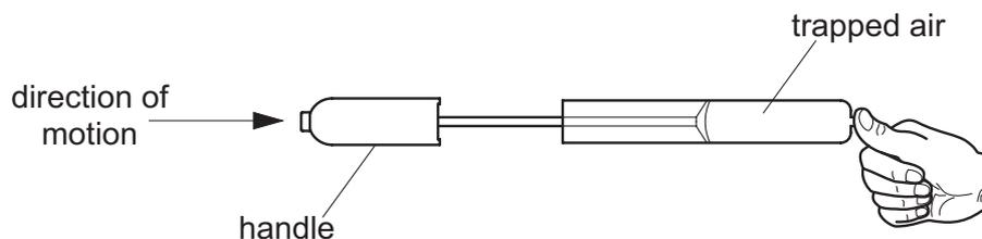
What happens to the pressure and to the volume of the trapped air as the pump handle is pushed in?
