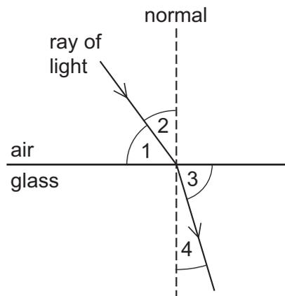
Which numbered angles are the angles of incidence and of refraction?
