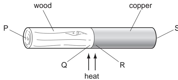
The rod is heated at the join in the centre for about a minute.
