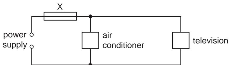
The current in the air conditioner is  $4.0\text{A}$  and the current in the television is  $6.0\text{A}$ .
