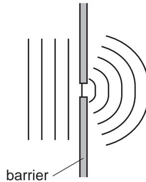
The waves spread out on the far side of the barrier.
