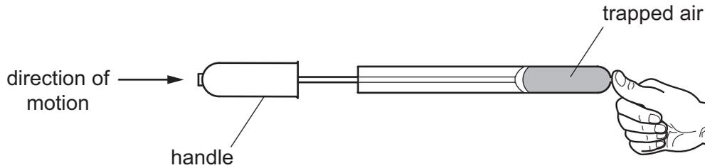
What happens to the pressure and what happens to the volume of the trapped air as the pump handle is pushed in?
