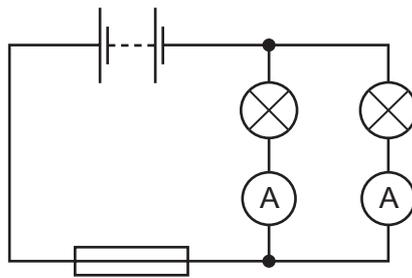
What is a suitable rating for the fuse in this circuit?
