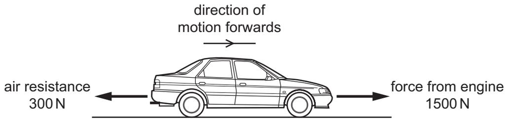
What is the size and the direction of the third horizontal force acting on the car?
