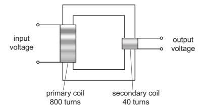
The input voltage is 240 V.
