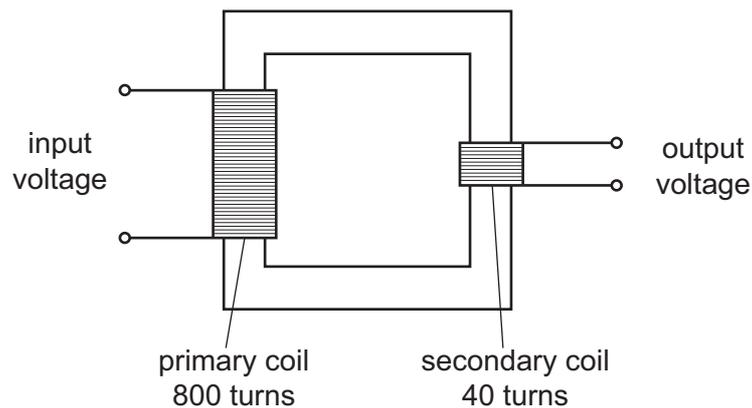
The input voltage is 240V.
