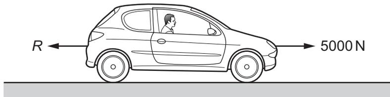
The car has a mass of 800 kg and an acceleration of  $1.0 \text{ m/s}^2$ .
