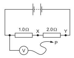
P is moved to point Y in the circuit.
