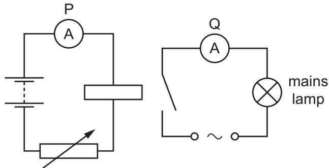
The variable resistor is used to vary the current in the relay coil. The mains lamp switches on when there is a large enough current in the relay coil.
