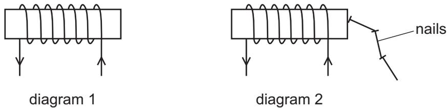
When there is no current in the coil, the nails drop off.
