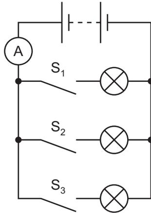
With only switch  $S_1$  closed, the reading on the ammeter is 0.04 A.
