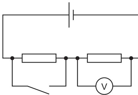
When the switch is open the voltmeter reads 1.5 V.
