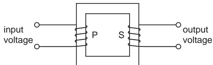
Which arrangement could be used to make the output voltage higher than the input voltage?
