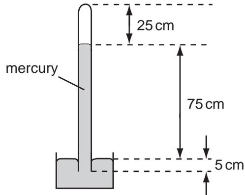
Which distance is used to calculate the pressure of the atmosphere?
