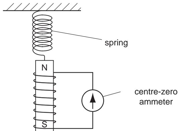
What does the ammeter show when the magnet vibrates slowly up and down?
