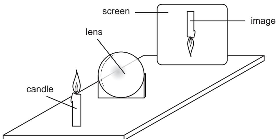
The screen and the lens are moved back and forth and various focused images are produced on the screen.
