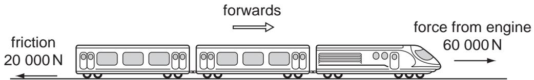
A force of air resistance is also acting on the train to give it a resultant force of zero.
