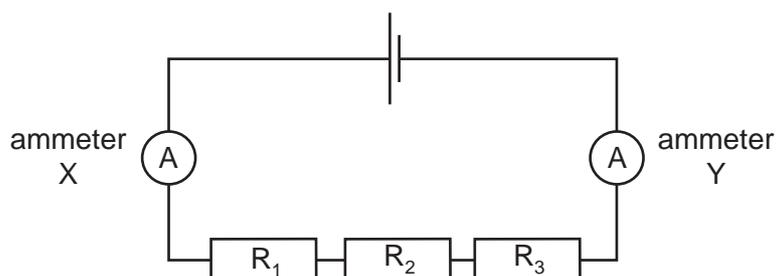
Which of the ammeters will show the current in resistor  $R_2$ ?
