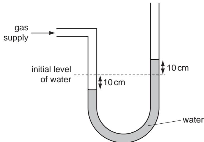
When it is attached to the gas supply, the water falls on the left side and rises on the right side. The difference in the levels of water on the two sides is now 20 cm.
