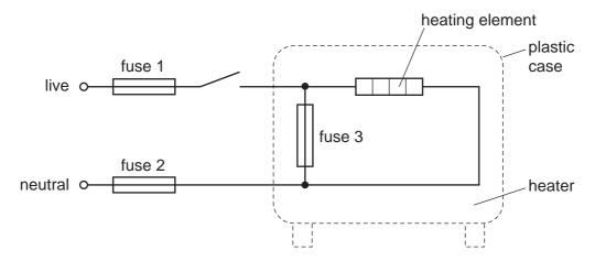
Which of the fuses are correctly placed?
