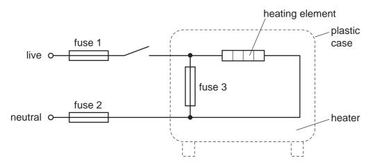
Which of the fuses are correctly placed?
