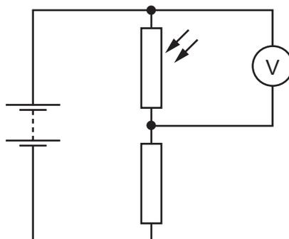
The brightness of the light falling on the LDR is increased.
