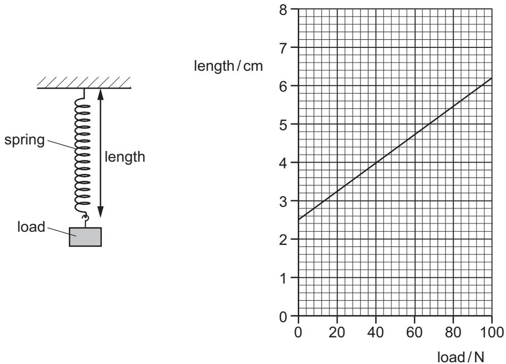
What is the extension of the spring when a load of 40 N is applied to it?
