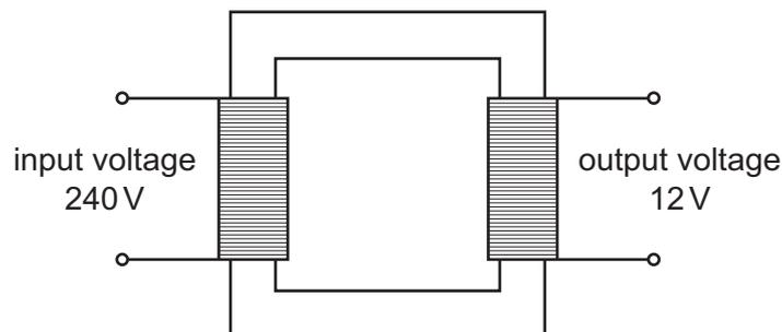
What is a possible pair of values for the number of turns in the primary coil and the number of turns in the secondary coil?
