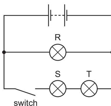
When the switch is open, which lamp or lamps are **not** lit?
