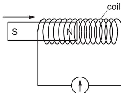
The needle of the galvanometer moves.
