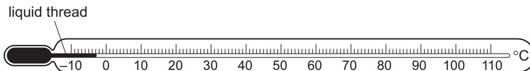
When the temperature of the thermometer rises, the changes produced cause the liquid thread to move to the right.
