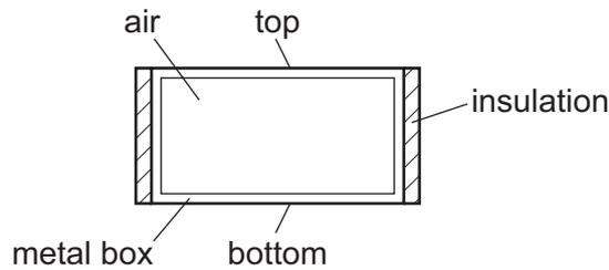
A scientist investigates the thermal conductivity of air. She measures how quickly thermal energy passes between the top and bottom of the box.
