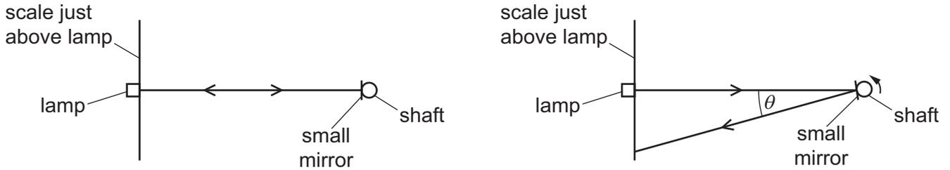
The beam from the lamp reflects from the mirror to give a small spot of light on a scale placed just above the lamp. The shaft and mirror rotate through  $1^\circ$ . The spot of light moves along the scale.
