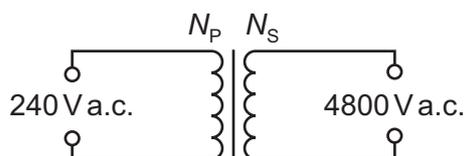
Which pair of coils would be suitable for this transformer?
