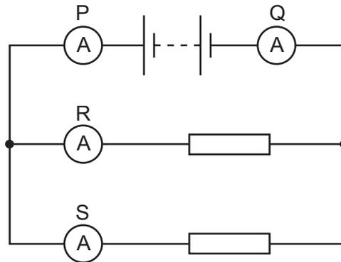
Which two ammeters read the largest current?
