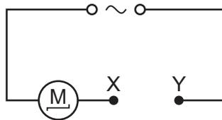
Which device needs to be connected between point X and point Y to prevent the wires from overheating if a fault in the motor causes the current to get too high?
