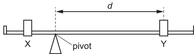
Which graph shows how the moment produced by load Y varies as the perpendicular distance  $d$  from the pivot changes?
